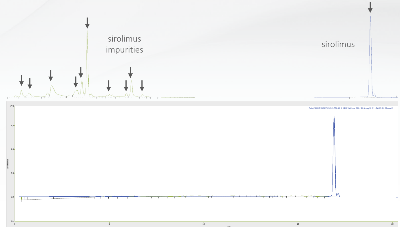
HPLC chromatogram of degraded sirolimus (green chromatogram) and intact sirolimus (blue chromatogram) – additional peaks indicate impurities and degradation products
